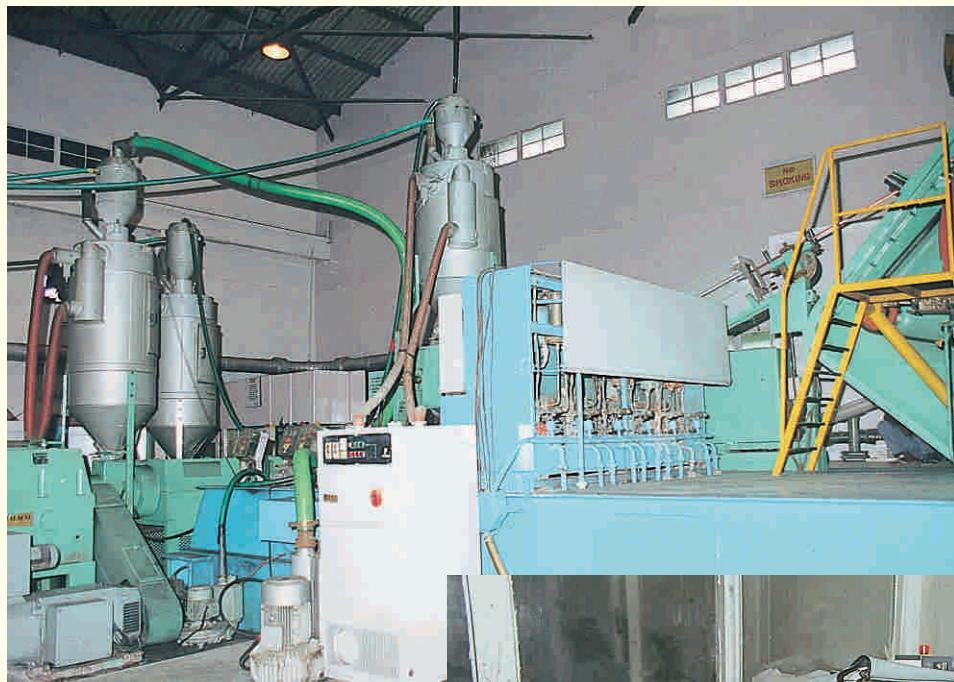
Continuous Catenary Vulcanising (CCV) Extrusion Platform
